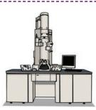
**Cryo-Electron Microscopy** Typically a transmission electron microscope is used to capture images of a rapidly frozen virus or sample, then computers create clear images of the molecular structure of the sample.
