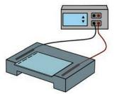
**Gel Electrophoresis** When charged by an electric current, molecules separate and move through a gel. Colored stains in the gel allow the molecule to be seen.
